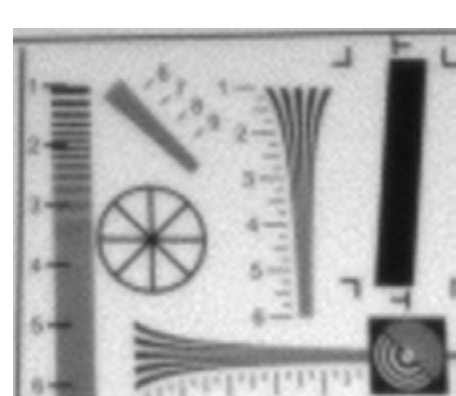
Figure 4: Top row) InVisage Spark P2 1.1 \mu\text{m} global shutter pixel imaging a resolution chart under pulsed 940 nm light. The smaller pixel size provides better spatial resolution. The right-hand panel shows a magnified view of the chart. Bottom row) A conventional silicon CMOS sensor with 3 \mu\text{m} global shutter pixels imaging a resolution chart under pulsed 940 nm light. The image has comparatively poor resolution and sharpness. The right-hand panel shows a magnified view of the chart.
