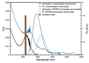
Figure 2. Absorption and luminescence spectra of (~10 mg/mL) PbS quantum dots prior to and following exchange to aqueous solution. Solid lines represent absorption spectra. Dashed lines represent photoluminescence spectra. Dark lines represent original OA capped PbS nanocrystals in toluene. Gray lines represent MTPEG-exchanged capped PbS nanocrystals in 20 mM HEPES buffer. Solid bar represents excitation wavelength used for PL spectra collection.
