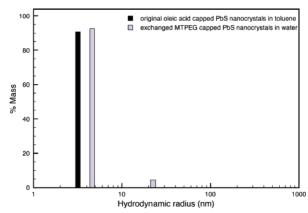
Figure 1. Dynamic light scattering measurements of hydrodynamic radius, by % mass modeled as solid Rayleigh spheres, of unexchanged PbS nanocrystals with oleic acid ligands (solid bars) in toluene, and PbS nanocrystals exchanged to having MTPEG ligands (shaded bars) in water.
