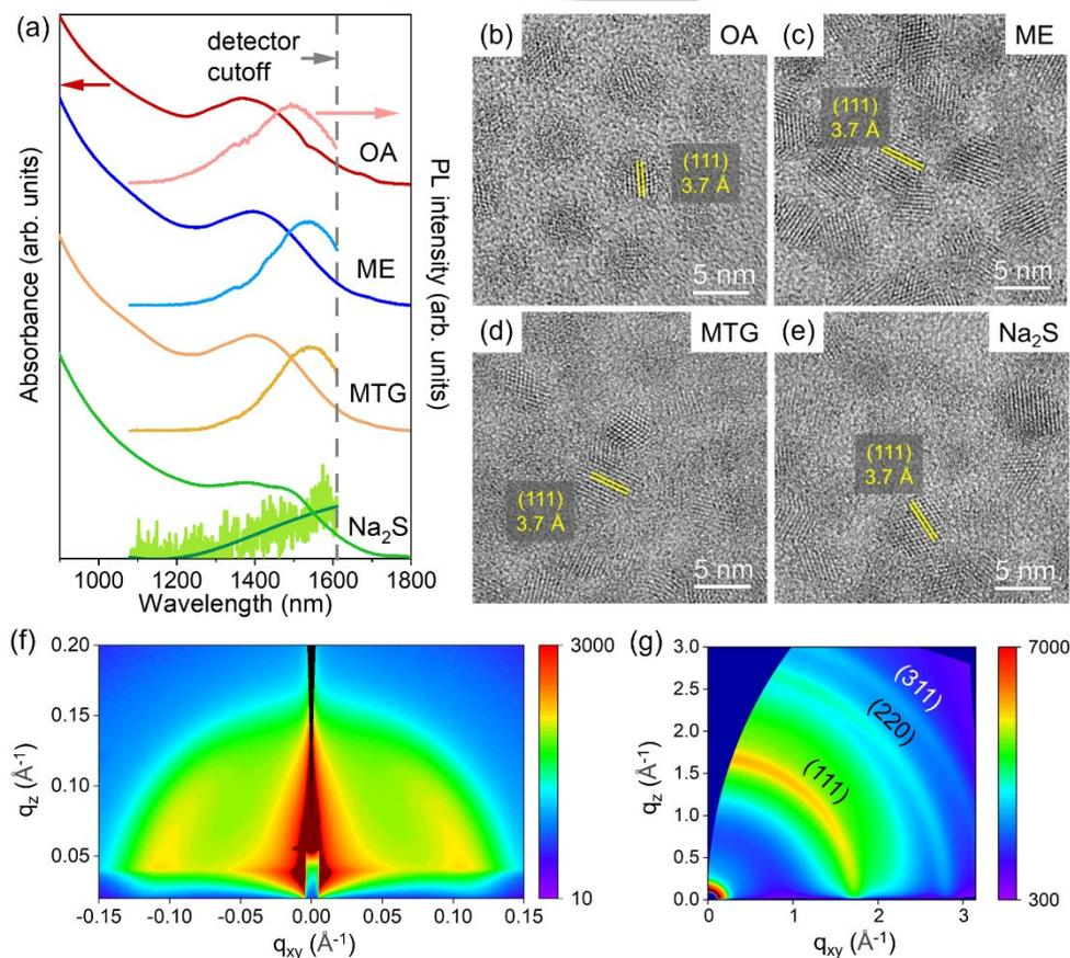
**Figure 3.** (a) Absorbance and PL spectra, and (b-e) high-resolution TEM images of InSb CQDs passivated with different ligands (OA, ME, MTG, or  $Na_2S$ ). The lattice spacings of 3.7 Å in (b-e) correspond to the (111) planes of InSb with zinc blende crystal structure. (f) GISAXS and (g) GIWAXS of ME-passivated CQDs.
