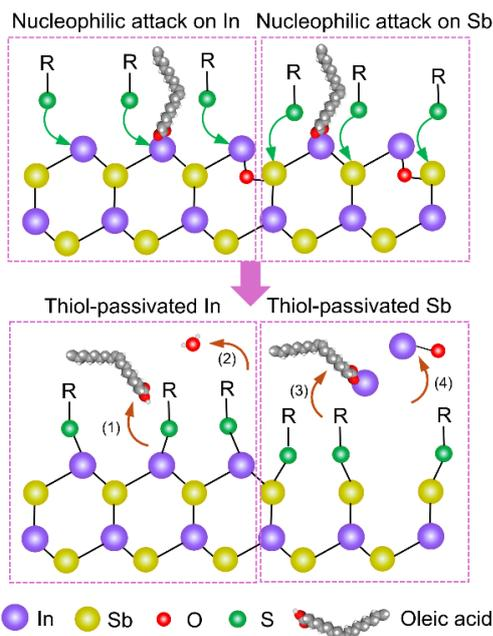
**Scheme 1.** Illustration of thiol-mediated surface reconstruction mechanism. Left: thiols attack the surface In atoms, leading to the detachment of (1) oleic acid and (2)  $O^{2-}$  anions that combine with free protons to form water. Right: thiols attack the surface Sb atoms, releasing (3) In-oleate and (4) In oxides.
